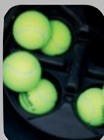
18. BALL FEEDER PLATE (INSIDE FEEDER POCKET)
